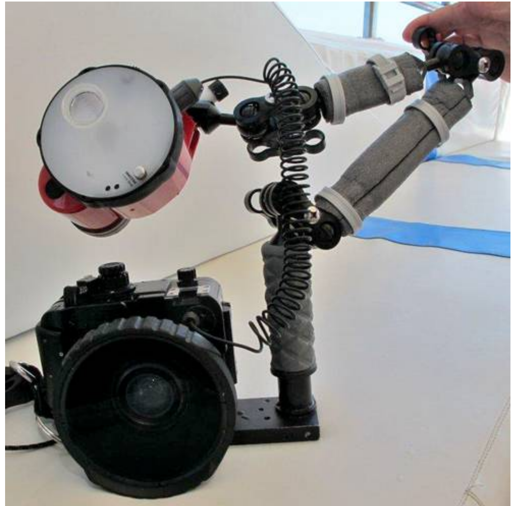
Caisson SEATOOL FIXG10 + grand angle + Canon G10 + Flash Inon D2000
